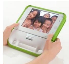
There are internal stereo speakers, as well as a stereo line-out jack. The microphone is built in, with a mic-in jack, which offers another unique feature: “sensor input” mode. The children can plug in any of a number of home-made data sensors, enabling them, for example, to turn their machines into thermometers or oscilloscopes.
