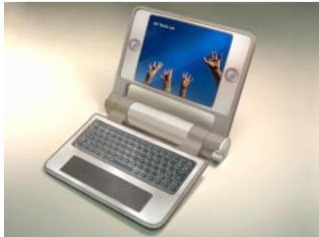
The existing design includes an innovative wind-up power source, runs on open source Linux software, and will be Wi-Fi capable.
